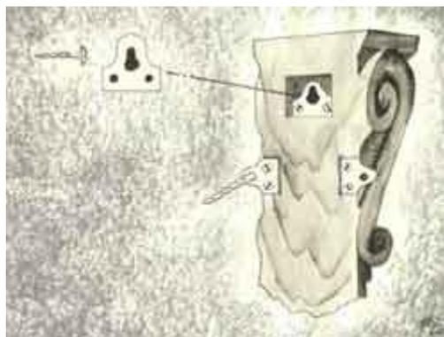
To fit these in a concealed manner, first pre-drill and fix the mirror plate to the back of the carving. Then offer up the work, mark fixing points and set plugs into the solid structure of the wall to take the mirror plate fixings.
